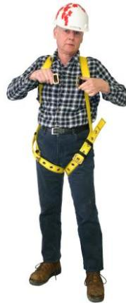
6. Now that all the straps have been fastened, your harness should fit snugly and allow you to have a full range of movement. Slide the plastic keepers against the buckles on the chest strap to ensure that your harness does not come out of adjustment. Put the ends of the leg straps through the fabric loops to keep them out of the way.
