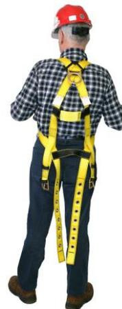
4. Making sure that the sub-pelvic strap is located under the buttocks, grasp leg straps from between your legs and connect to the opposite ends of the shoulder straps at the front of the hips.
