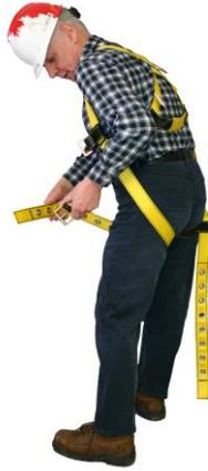
5. Position your chest strap roughly six inches from the top of your shoulders on the front of the harness and connect. Tighten your chest strap enough to keep the shoulder straps taut and prevent them from slipping off the shoulders.
