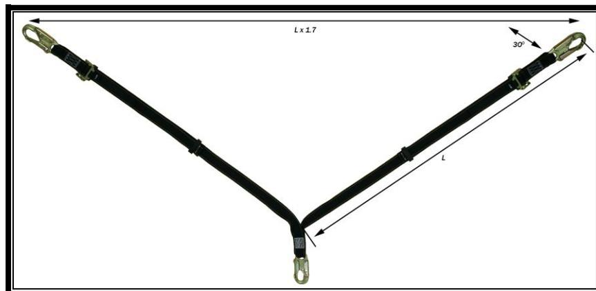
The 'Y' or Bypass lanyard is designed for only momentary attachment to two (2) anchorages. Attachment of the two legs to separate anchorages, simultaneously for prolonged periods of time, could result in serious overloading of the lanyard if the distance between the anchorages exceeds 1.7 times the lanyard length, or if the angle between the lanyard leg and the horizontal is less than 30° (degrees).
