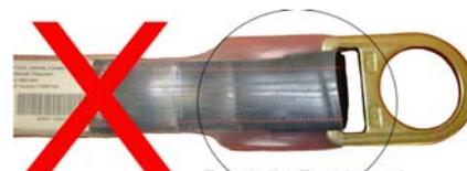
Partially Deployed HLL Energy Absorber
