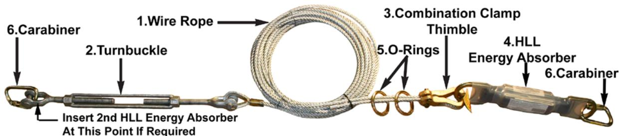
The horizontal lifeline system should be unpacked and unrolled to ensure that the cable is not kinked before or during installation. The system is fully assembled as shipped but the bolts are not tightened on the combination clamp. The turnbuckle should be adjusted so that it is at its maximum length.
