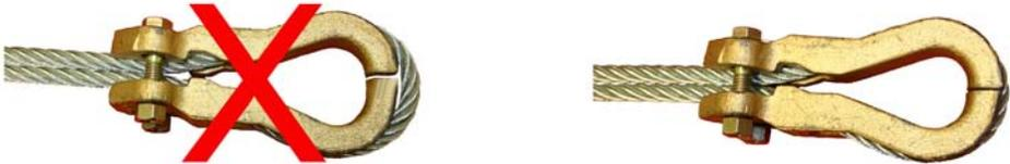
Once the approximate adjustment has been made, the bolts on the clamp should be torqued to 40 ft / lb.
