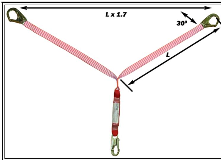
If the distance between the anchorages exceeds 1.7 times the lanyard leg length then a horizontal lifeline should be used to facilitate the point-to-point transfer.
