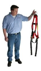
3. Slip shoulder straps onto your shoulders so that the D-ring is now located between the shoulder blades in the middle of your back.
