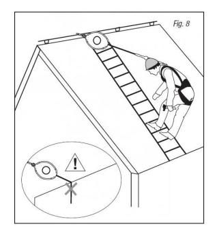
WARNING For all assembly configurations: The anchoring to the structure must allow self-alignment of the SRD under the effect of the force exerted on the web/cable. Mount the SRD with the carabiner inserted through the built-in swivel at the top of the unit. (Figure 10).
