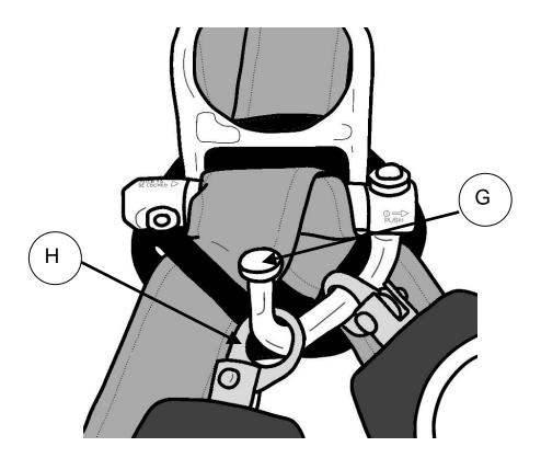
8.7. Close the connector by moving the webbing away from the slot and pushing on the locking bar until it clicks. The indicator will be RED if the carabiner is not locked properly.
