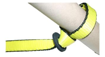
Follow the same steps to attach the other end to a secure anchor point or another section of hose. After both loops are secured, move them away from each other so there is no slack in the whip check.
