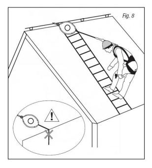
7.4.4. If the user is working on a sloped area, the length of the SRD must be adapted to the dimensions of the working area (Figure 9).
