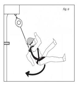
WARNING The user must not exceed an angle of 30° and never move away from the vertical axis of the SRD for more than 10 ft. (3 m) (Figure 7).
