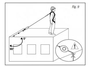
WARNING For all assembly configurations: The anchoring to the structure must allow self-alignment of the SRD under the effect of the force exerted on the wire rope. Mount the SRD with the carabiner inserted through the built-in swivel at the top of the unit. (Figure 10).
