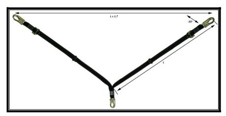
The 'Y' or Bypass lanyard is designed for only momentary attachment to two (2) anchorages. Attachment of the two legs to separate anchorages, simultaneously for prolonged periods of time, could result in serious overloading of the lanyard if the distance between the anchorages exceeds 1.7 times the lanyard length, or if the angle between the lanyard leg and the horizontal is less than 30° (degrees).
