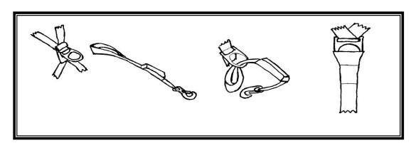
The lanyard should be attached to the D-ring on the dorsal extension, in accordance with the regulations in the jurisdiction in which the equipment is being used.
