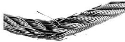
Fatigue (Undersized Sheave)
