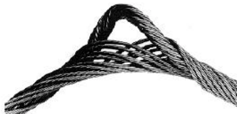
Figure 10, Core Protrusion, Indicating Shock Loading
